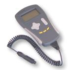
The Curtis Model 1311 Handheld Programmer is ideal for setting parameters and performing diagnostic functions.
